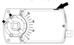
3. Place the stem adapter on the valve stem and make sure the arrow on the adaptor is aligned with the arrow on the valve stem.
