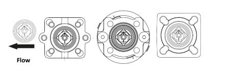
4. Place the plastic support and fix it through the 4 screws according to the valve type. Then, place the actuator (in position 0°), block it behind and fix the stem adaptor. Assembly the lever.
