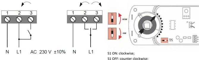
With factory settings (see picture above, S1 OFF), if wires 1 and 2 are connected the valve opens; if wires 1 and 3 are connected valve closes.
