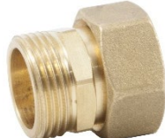
1007MC – Douille \frac{3}{4} " F sf.x \frac{3}{4} "M portée plate
