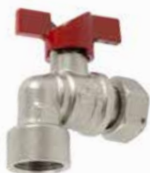
F (free nut) x F angle ballvalve for water meter. Anti-legionella ball with additional bore on the bottom to avoid water stagnation in the space between the ball and the body. Red butterfly handle. Nickel plated.
