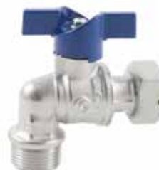
F (free nut) x M angle ballvalve for water meter. Anti-legionella ball with additional bore on the bottom to avoid water stagnation in the space between the ball and the body. Blue butterfly handle. Nickel plated.
