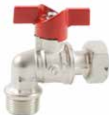
F (free nut) x M angle ballvalve for water meter. Anti-legionella ball with additional bore on the bottom to avoid water stagnation in the space between the ball and the body. Red butterfly handle. Nickel plated.
