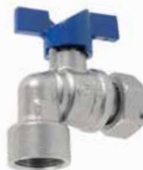
F (free nut) x F angle ballvalve for water meter. Anti-legionella ball with additional bore on the bottom to avoid water stagnation in the space between the ball and the body. Blue butterfly handle. Nickel plated.
