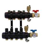
Modular manifold made of PA66/brass, pre-assembled with terminal set, distribution valve, return valve 1" F with pocket for thermometer and thermometer (T39P/80).
