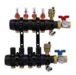
Modular manifold made of PA66/brass, pre-assembled with terminal set, flowmeter, distribution valve, return valve 1" F with pocket for thermometer and thermometer (T39P/80). Flow rate: from 1 1/min to 5 1/min.
