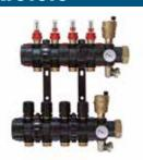
Modular manifold made of PA66/ brass, pre-assembled with terminal set (thread Ø 1" F flat end), thermometer (T39P/80) and flowmeter. Flow rate: from 1 l/min to 5 l/min.
