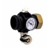
Terminal set in synthesis material PA66 and brass composed of a "T" terminal, a manual air-vent, a drain and a thermometer. Available with 1" or 1 1/4" flat end inlet thread.
