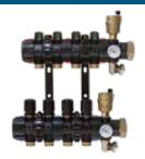
Modular manifold made of PA66/ brass, pre-assembled with terminal set (thread Ø 1" F flat end) and thermometer (T39P/80).
