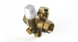
Adjustable thermal balancing valve for sanitary hot water recirculation systems, made by lead free corrosion resistant brass. PN16, Max working temperature 90°C. Temperature setting range:  $35^{\circ}$ -  $60^{\circ}$ C. Kv max: 1,80. Available connections F x F or M x M (TB20/2).
