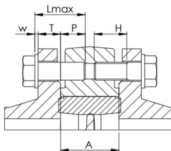
Suggested length in case the valve is installed between steel flanges EN1092-1 type 11 PN16 and PN10, with DIN125/ISO7089 washers. Always verify the screw length according to installation requirements.
