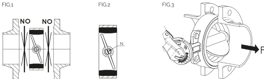
The valve allows the dismantling of the pipes downstream, for pressures below 6 bar. For end of line installation:
