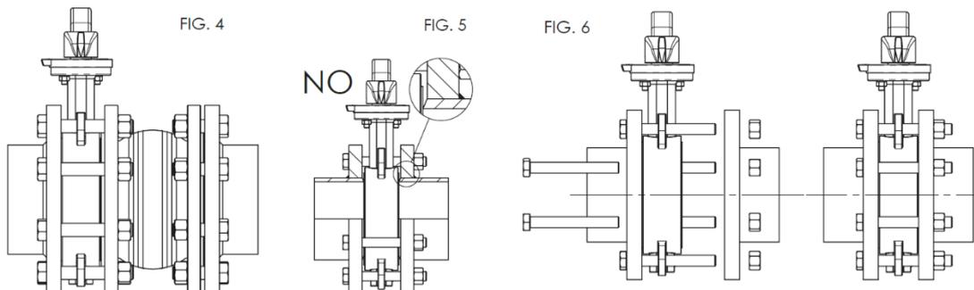
Turbulences of the fluid might increase erosion and reduce the life-cycle of the valve. Install the valve at a distance of at least 1 x DN upstream and 2-3 x DN downstream, away from fittings or bends.
