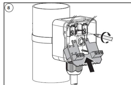
Wiring according to the available control unit as shown by figures 9a and 9b. Possible reversal of cables at the 24 V and 230V control units damages the humidity sensor.
