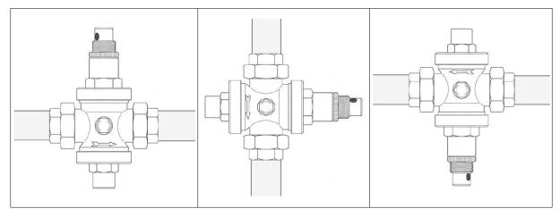
Please check that the flow direction is concurrent to the arrow on the reducer body. Commissioning and pressure set-up is done by rotating the brass spring holder on the top; to do it (see pictures below), loosen the plastic lock ring, turn the spring holder using a screwdriver (clockwise to increase outlet pressure, counter clockwise to decrease outlet pressure), tighten the plastic ring.
