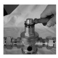
In order to set the system correctly, it has to be closed and a manometer M500P (not included) has to be installed.
