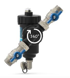
A specific feature of EvoMAGic 103 series is the orientable connection: despite the dirt separator has to work vertically, the 360° orientable connection allows the installation on different pipe direction. It can be installed on vertical, horizontal or tilted pipes. Installation requirements must be observed. Refers to specific INSTALLATION section.
